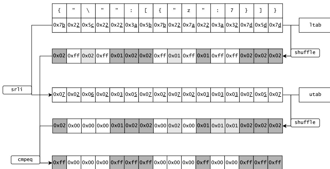
Figure 4.1: JSON document classified using the structural classifier’s ltab and utab lookup tables.
